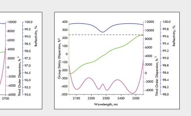
Infrared dispersive mirrors with negative GDD: PC1741 (left) and HD1501 (right).
