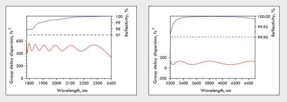
Infrared dispersive mirrors with positive GDD: IR1402 (left) and HD1715 (right).
